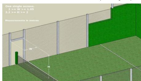
1) With one lateral access per side the opening must be a minimum of  $1.05 \times 2.00$  metres and a maximum of  $2.00 \times 2.20$  m (See diagram).
