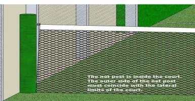
The outer side of the net posts should coincide with the lateral limits of the court, (opening, entrance or metallic fence). They may be circular or square but must have rounded edges.
